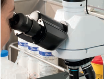
Routine microscope die-cast frame, with high stability and ergonomics, for transmitted light observation.
