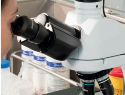
Routine microscope die-cast frame, with high stability and ergonomics, for transmitted light observation.
