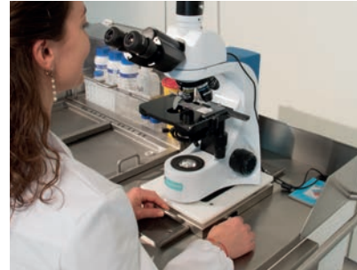
Adjustable microscope sleigh for ergonomic movement forward-backward
